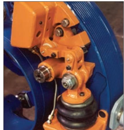
Air bag canister tool tensioning system
