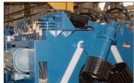
Pneumatic tensioning of feed rolls
